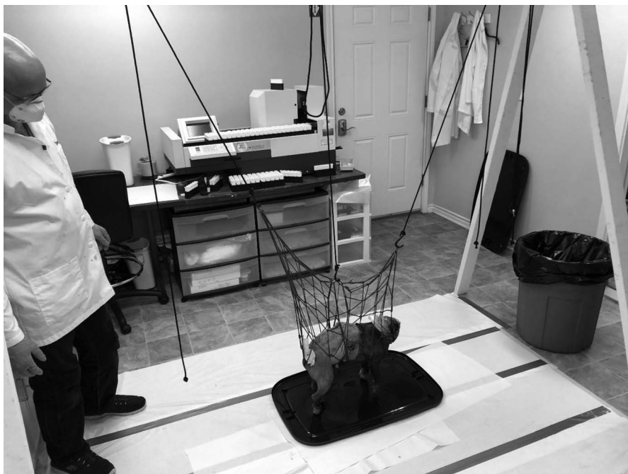
Fig. 2. Cadaver suspended in position for dose rate measurements.
