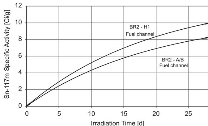
**Fig. 3.**  $^{117\text{m}}\text{Sn}$  yield for 200 mg 92%  $^{117}\text{Sn}$  enriched targets in the BR2 high-flux reactor.
