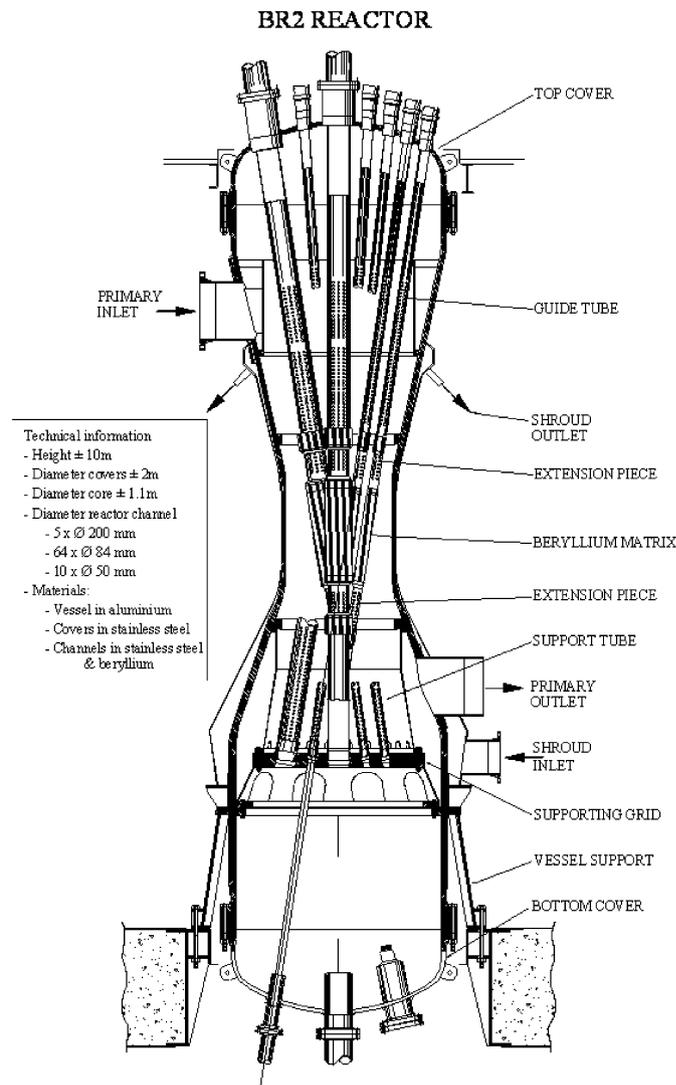
Fig. 1. BR2 high-flux reactor.
